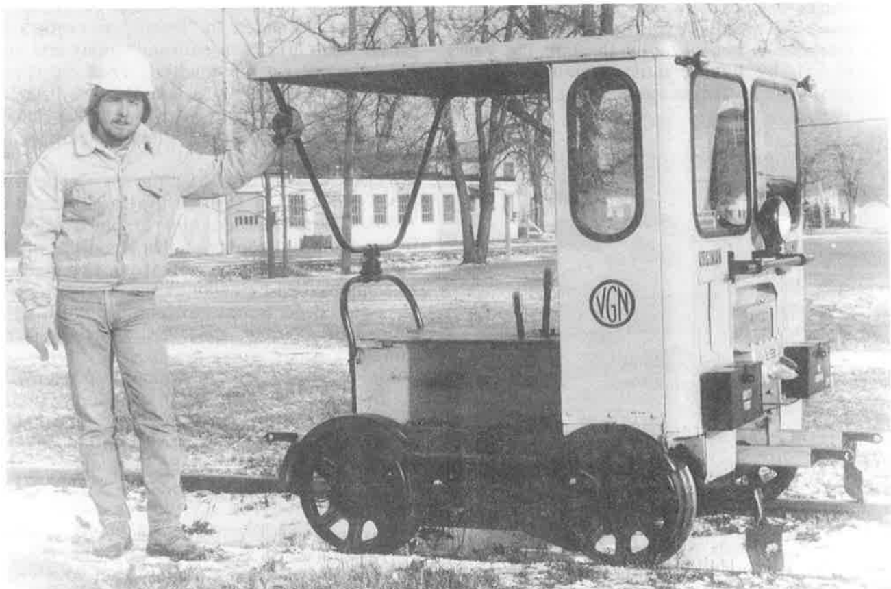
NARCOA member Jeff Mast poses momentarily by his ex Virginian Railway Fairmont M-19 during a winter work session on the Southern Michigan Railroad in December, 1986. Photo by Jeff Mast
