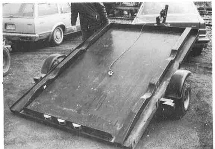
Fred Furminger uses a stock snowmobile trailer that is slightly "beefed up". Fred uses the tilt feature to load and unload his car with a tongue-mounted winch. The wooden "rails" have indentations to keep the car from shifting (even though it is tied down with cargo straps).
