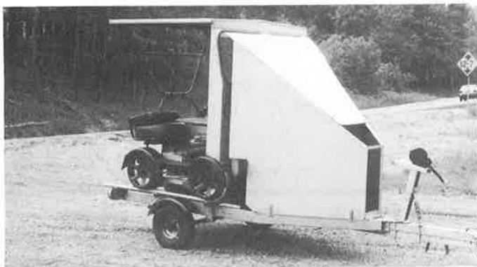
Dick Ray has modified this boat trailer for motor car use. In addition, he has installed a removable wind deflector to minimize wind drag. The trailer will accommodate either an M-9 or M-19 size car.
