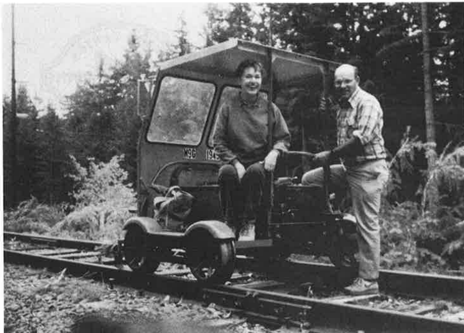
NARCOA members Mary and Roger Sackett operate this beautifully restored ex Northern Pacific Fairmont M-9, Series G car in the Pacific Northwest. Photo By Roger Sackett
