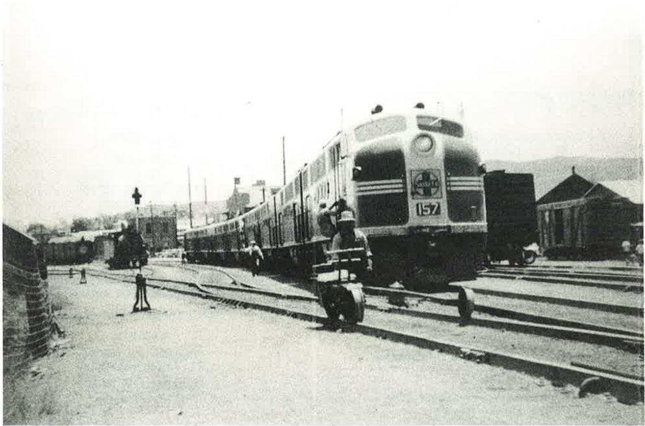
Forty years ago, the Santa Fe still had Electro-Motive FT freight diesels on its roster, as well as a few Sheffield velocipedes. In the view above, at Prescott, Arizona, recorded by the late Cecil Hommerding, we see a maintainer pause long enough for his picture to be taken before continuing on with his work of filling kerosene switch lamps (note the kerosene can on the tool tray of the velocipede). Left and Below- These two photos of a similar vintage show a Fairbanks-Morse gang car and motor car house in New York Central's Ft. Wayne, Indiana yards, on the old Ft. Wayne & Jackson Railroad.
