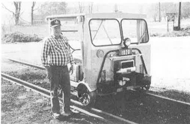
Red's "new" number 1020 is an ex Illinois Central M-19, formerly used by a signal maintainer.
