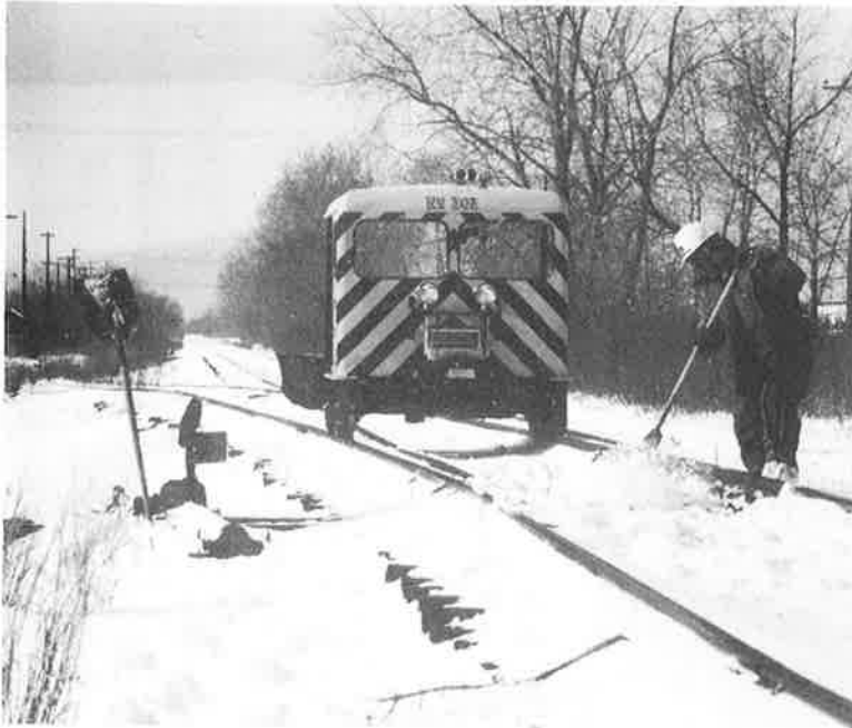
Fred Furminger uses his ex Chesapeake & Ohio Fairmont M-9 track car, the #303 for maintenance duties on the newly formed Depew, Lancaster & Western Railroad, a new short line in the Buffalo, New York area.
