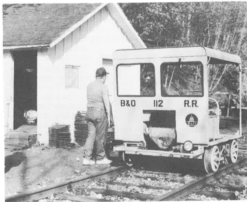
John Mowrer's Fairmont S2H is shown at the tool shed at Muddy Creek Forks on the Maryland and Pennsylvania RR. The car was built on July 11, 1949, for the B&O RR, and has a Kalamazoo cab, typical of B&O cars, and a one-cylinder RQD engine. Delivery was made to the B&O at Ravenna, Ohio, in 1949. To the left of the car is Mike Billet, who restored the car in 1992, and Wade Monn is standing beside the car.
