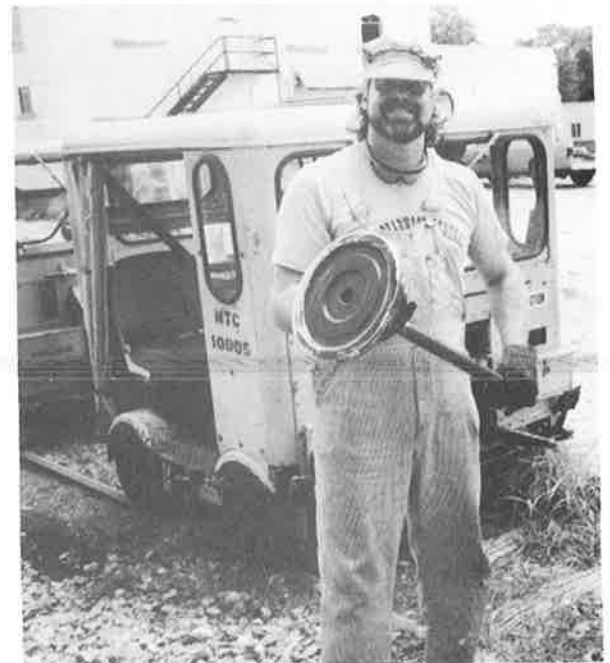
John Mowrer's Fairmont S2H is shown at the tool shed at Muddy Creek Forks on the Maryland and Pennsylvania RR. The car was built on July 11, 1949, for the B&O RR, and has a Kalamazoo cab, typical of B&O cars, and a one-cylinder RQD engine. Delivery was made to the B&O at Ravenna, Ohio, in 1949. To the left of the car is Mike Billet, who restored the car in 1992, and Wade Monn is standing beside the car.
