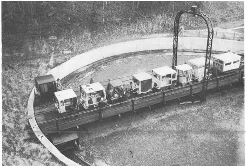
Several cars at a time were turned on the turntable at the end of the Western Maryland Scenic RR line in Cumberland, Maryland, in December 1991.
