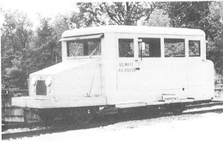
At left is a photo of a railbus built by the Crane Railroad Shops at the Crane Naval Surface Warfare Center in Indiana. Still in use today, it is powered by a six-cylinder Ford engine.
