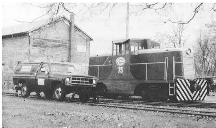
Above, Bob Schuknecht's GMC hy-rail pickup and the Southern Michigan Railroad's GE 44-ton center cab #75 (ex-Western Maryland 75), seen here in the Clinton yard, fall of 1996.
