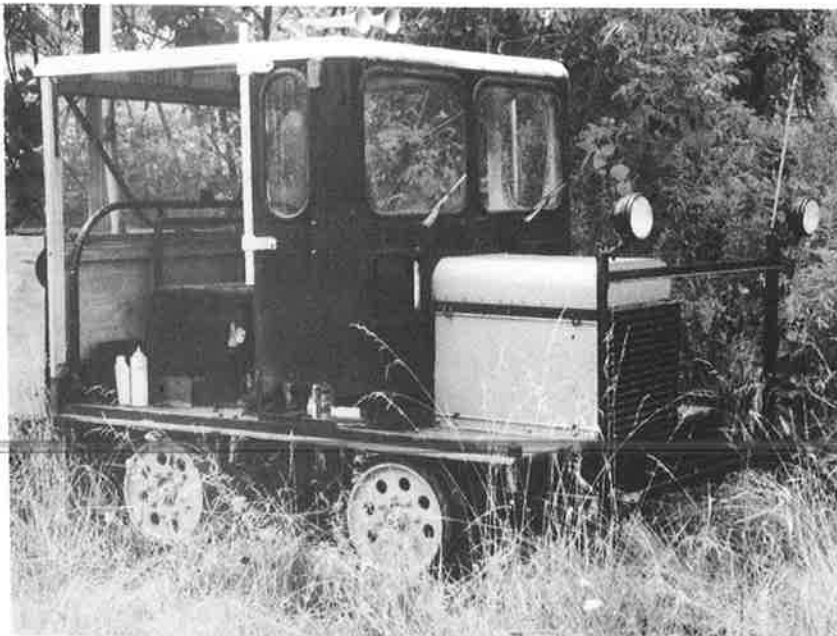
At left, an A series car, modified with an M series cab, on Ohi-Rail, September 3, 1995.
