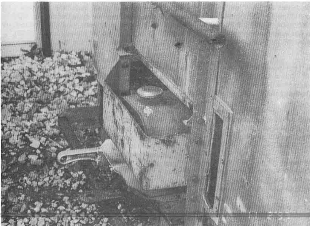
Above, a picture of the fuel tank guard installed on an MT14 by the Canadian National Railroad.
