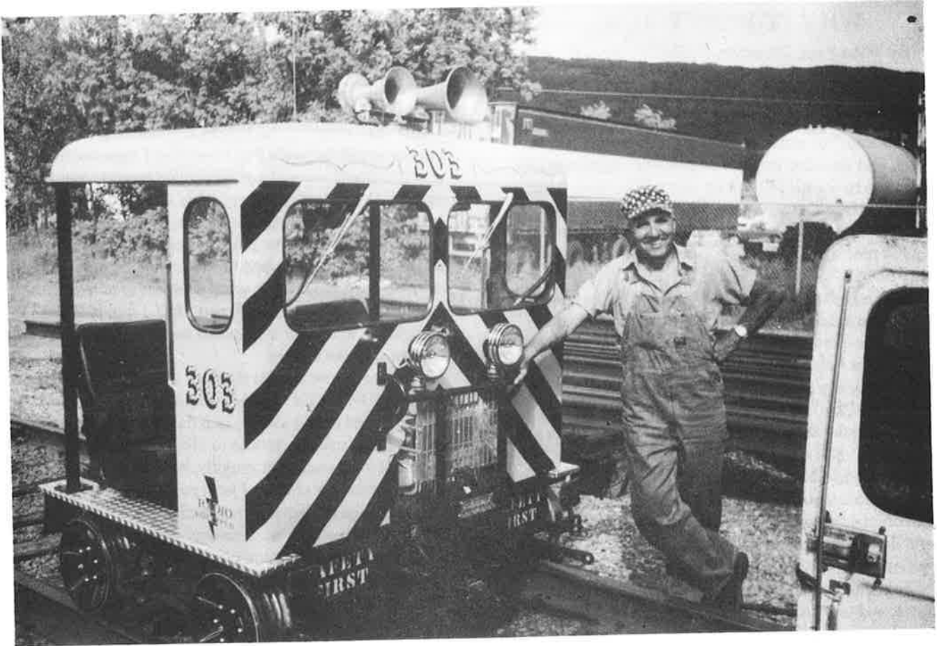
(Below) Photo by Doris Hurtig: Mt. Washington Cog RR (NH) speeder, June 22, 1988; Bombardier snowmobile engine; snowmobile machinery; Fairmont control panel.
