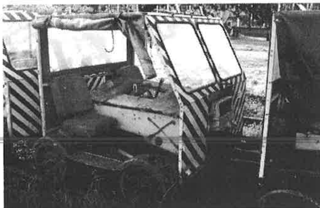
M19 FZ63s here await disposal at Islington workshops in Australia in 1992. Many have been rebuilt over the years, replacing aluminum frames with steel and failed motors with whatever was at hand.
