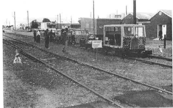
Cars at a speeder meet at Mount Gambier in South Australia. All cars here are broad gauge—63"—and are in order: A5, ST2H, M19F, ST2H, M19F, ST2H.
