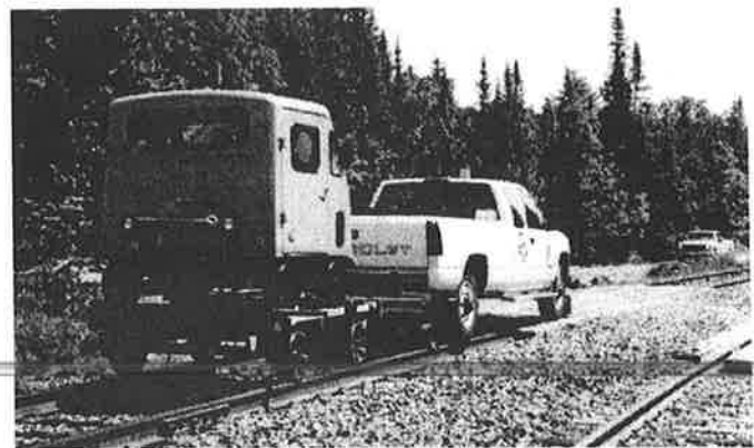
Gary Greenwood's Woodings Railcar suffered a frozen transmission during the July 26-29, 1999, excursion on the Algoma Central. As the rear axle was locked up, the car was loaded on a push car by the railroad and hauled back to Sault St. Marie. STAN CONYER PHOTO
