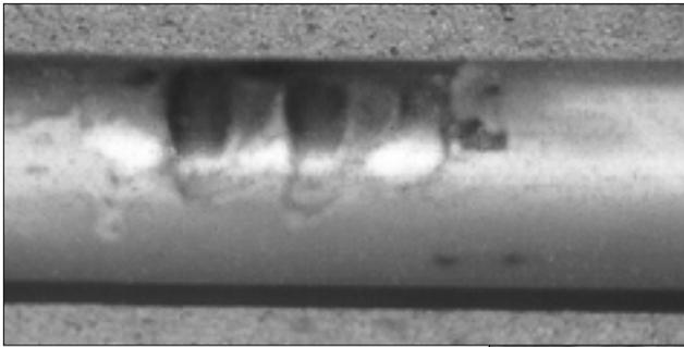
Also in the November/December 2000 issue was Tom's warning about excessive wear on brake shafts caused by drive chains. These photos show slack chains can wear through a shaft, allowing it to bend or break during brake application.
