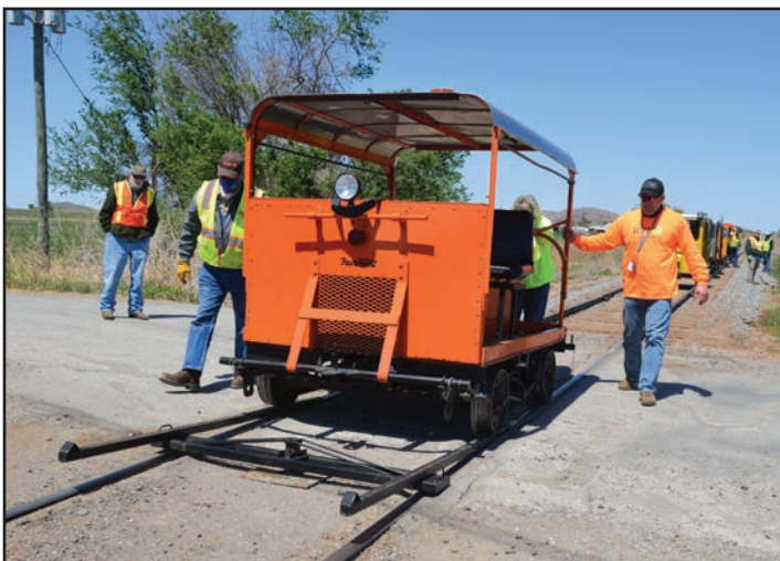
Don Kendall engineered the turntable for his A car. The truss mounts on the back of his car and acts as a bumper!
