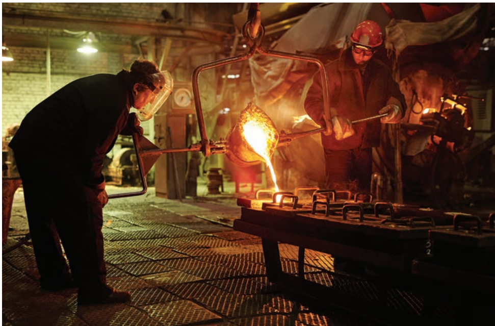
Molten iron being poured in New England at Enterprise Casting; photo courtesy of Eliza Trauger at www.Carefree-Creative.com
