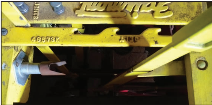
A piece of copper tubing cut in a 'V' shape was added over the starter switch to capture the lever. V bracket on right keeps the lever from going too far forward.
