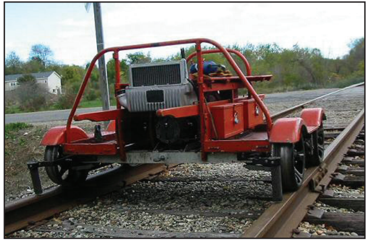
My M9-C It runs off a dry battery - no generator or alternator.
