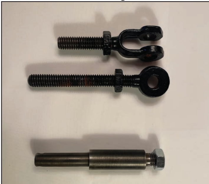
Above, a Fairmont yoke and eye bolt with original 12 TPI jam nuts, and below a NOS pivot stud with a modern 13 TPI half nut
